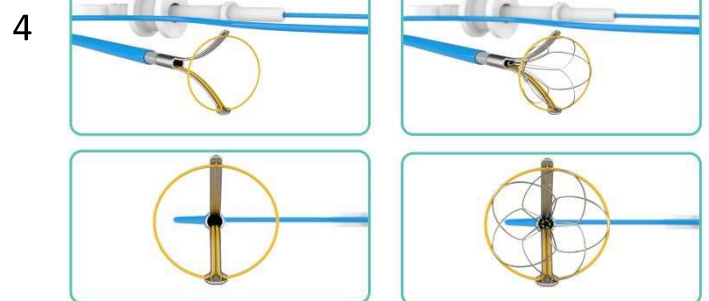
Figure 4. The forward-facing cold snare polypectomy device concept features a braided wire shape memory snare that is expanded in a plane perpendicular to the length of the catheter. The snare may be expanded with prongs that are extended from the catheter. The snare may be contracted by pulling on a purse-string feature.
