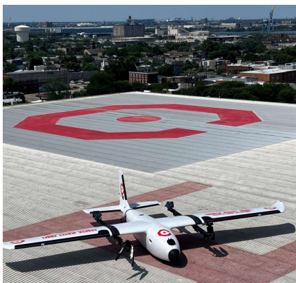
Figure 1. Photo of the Jersey Angel Prototype. With vertical takeoff and landing, deployment can happen in seconds almost anywhere.
